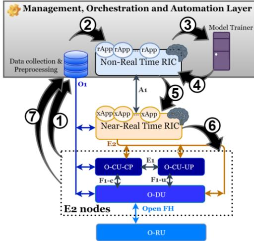
Fig. 4. ML-based workflow executed at the O-RAN
